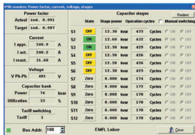
Configuration and remote indication of the measuring values via RS232 interface with EMR 1100.
